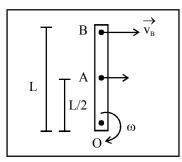
$v_{_{B}} = \omega L$  and  $v_{_{A}} = \frac{\omega L}{2}$ , with directions as shown in figure.
